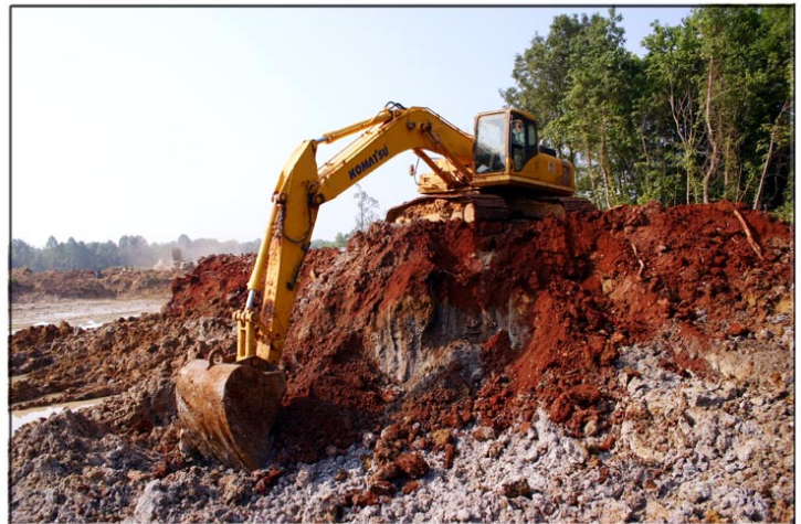
Stanley's Komatsu PC300LC trackhoe w/ Topcon's LS-B3 laser indicate system
