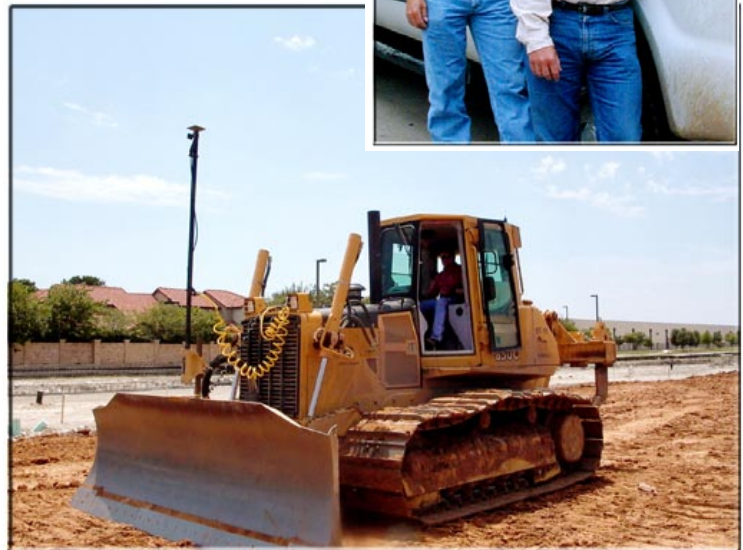
L & K's John Deere 850C w/ Topcon's SystemFive 3D-GPS+ automatic machine control
