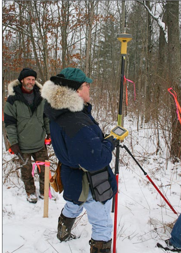
Using the FC-2000 controller and GR-3, Lang's crew can quickly and accurately move from data collection to well-staking.
