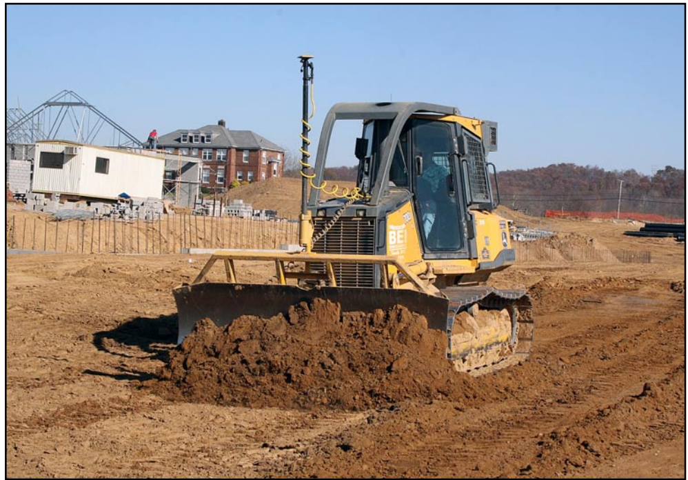
Brown estimates that Topcon's 3D-MC 2 system will probably knock four to six weeks off the project length, largely because of gains they made in final grading.
