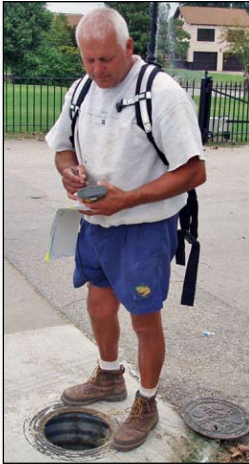
Don Shope uses a Topcon GMS-110 GPS unit and FC-100 data collector to record information on a water meter location for the city of Tulsa, Oklahoma. Shope is an employee of Keystone Plumbing, a subcontractor to W. N. Couch.
