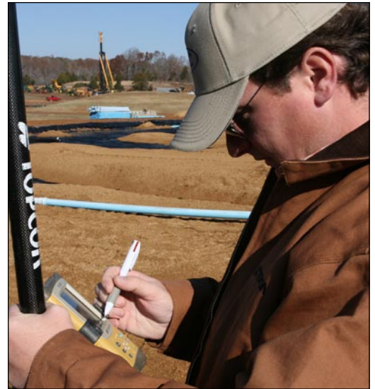
BOTTOM: Ellsworth checks settings on the Topcon satellite receiver rover unit.
