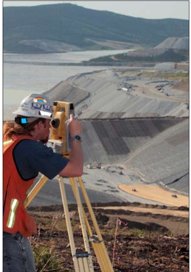
Surveyors at an Alaska gold mine track material extraction safely and productively from a distance using the IS imaging, scanning and robotic total station.
