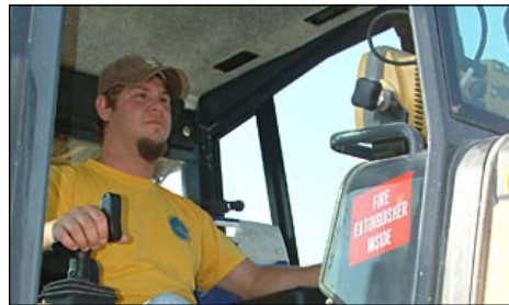
(TOP LEFT AND RIGHT) Lake County Grading's Joe Gore operates a John Deere 850 dozer outfitted with Topcon 3DMC that accesses PSG Net for real-time GNSS guidance at the fairgrounds. (BOTTOM RIGHT) Ruben Cuevas, chief surveyor of Lake County Grading Co., uses a HiPer rover in the networked area.
