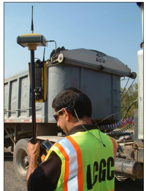
(TOP LEFT AND RIGHT) Lake County Grading's Joe Gore operates a John Deere 850 dozer outfitted with Topcon 3DMC that accesses PSG Net for real-time GNSS guidance at the fairgrounds. (BOTTOM RIGHT) Ruben Cuevas, chief surveyor of Lake County Grading Co., uses a HiPer rover in the networked area.
