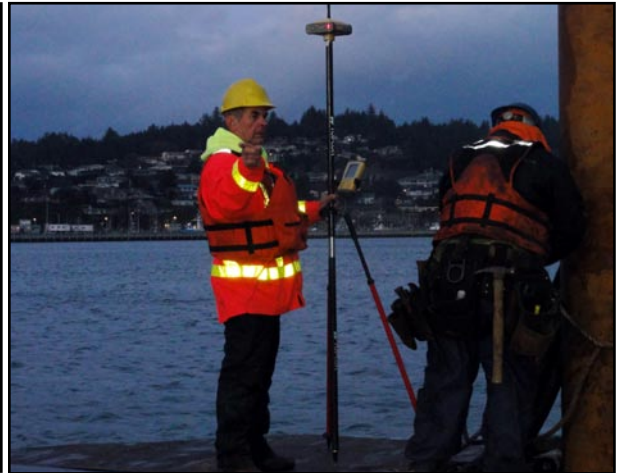
LEFT: WCC set up a Topcon HiPer Lite+ base station on shore. RIGHT: WCC's Greg Damms using HiPer Lite+ rover.
