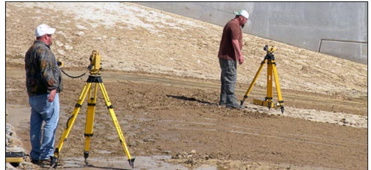
Left : Several million points were collected with the GLS-1000. Top: Topcon total stations, auto and digital levels were used for the project.
