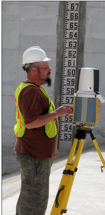
Left : Several million points were collected with the GLS-1000. Top: Topcon total stations, auto and digital levels were used for the project.
