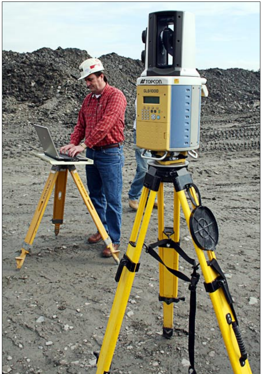
Lynell Early, vice president, PERC Engineering, collects data on stockpiles using a laser scanner.
