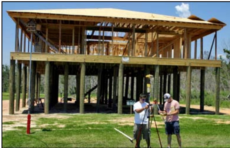
Dunivant and Baxter prepare to shoot features of a typical coastline residence. Topcon's HiPer+ rover is connected to the CORS site with a cellular modem
