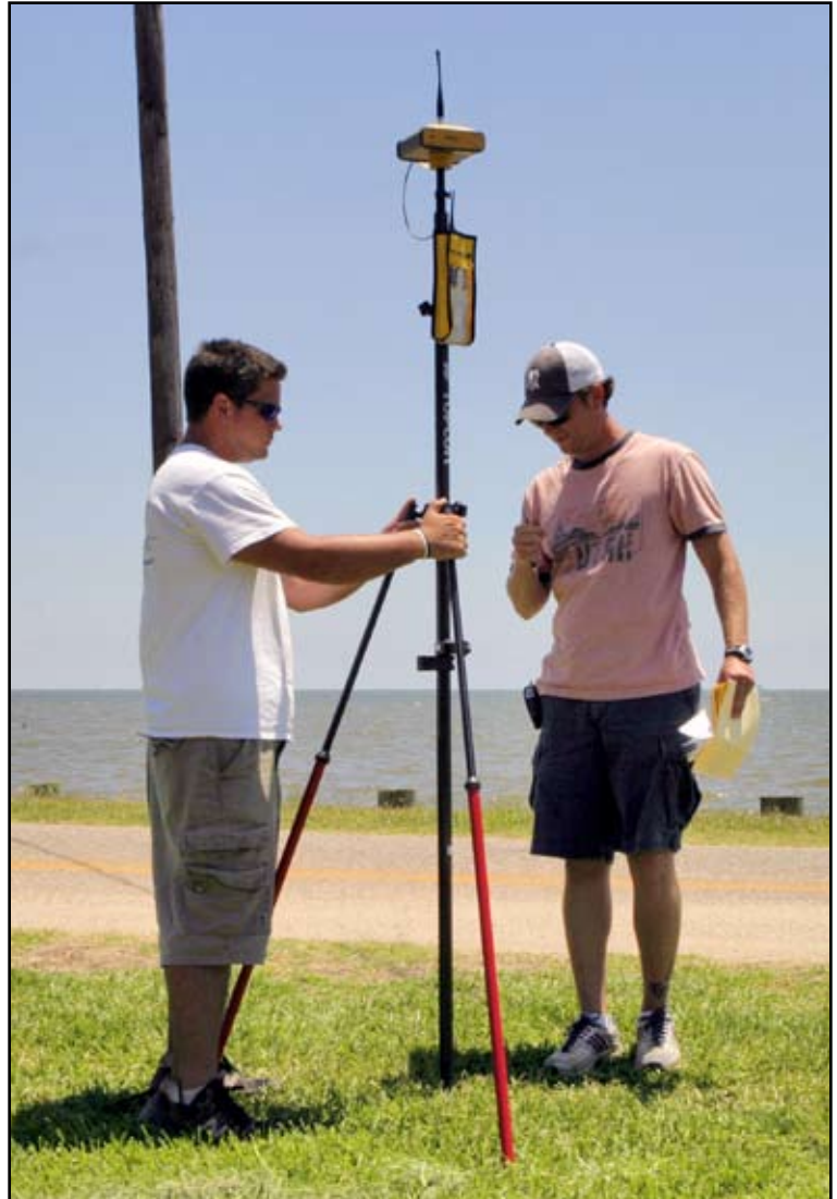
Ricky Dunivant and Clayton Baxter set an elevation reference hub on the edge of Mobile Bay, 17 miles from Topcon's CORS site near the home office.
