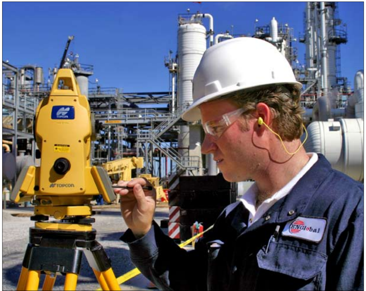
Ben Sherrod shoots an elevated structure with Topcon's GPT-7001i
