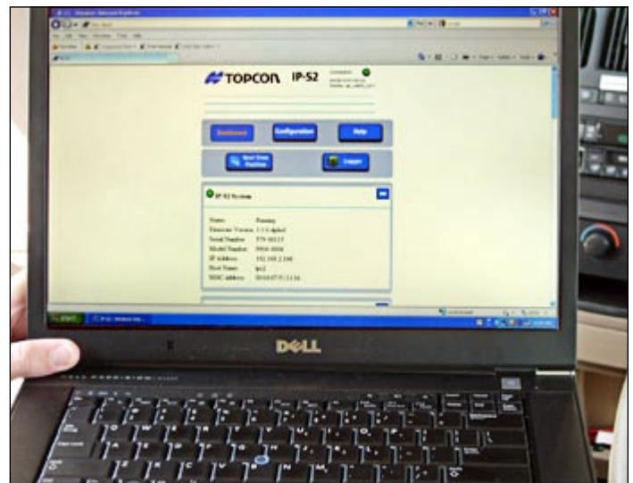
BELOW: The IP-S2 utilizes a Web browser; an Internet connection is not necessary during data collection.
