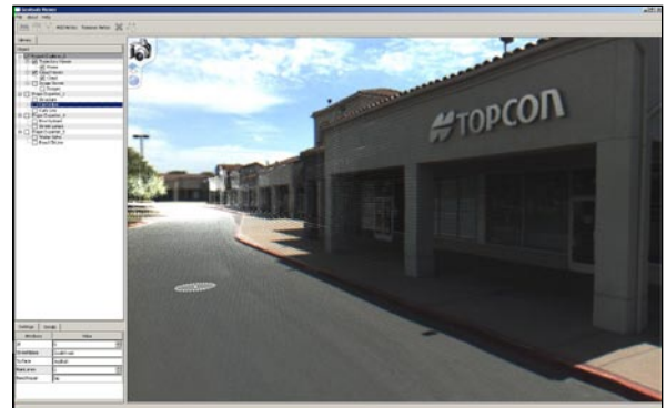
Integration of LIDAR point cloud data with digital imaging allows user to obtain coordinate measurement of objects and surfaces.
