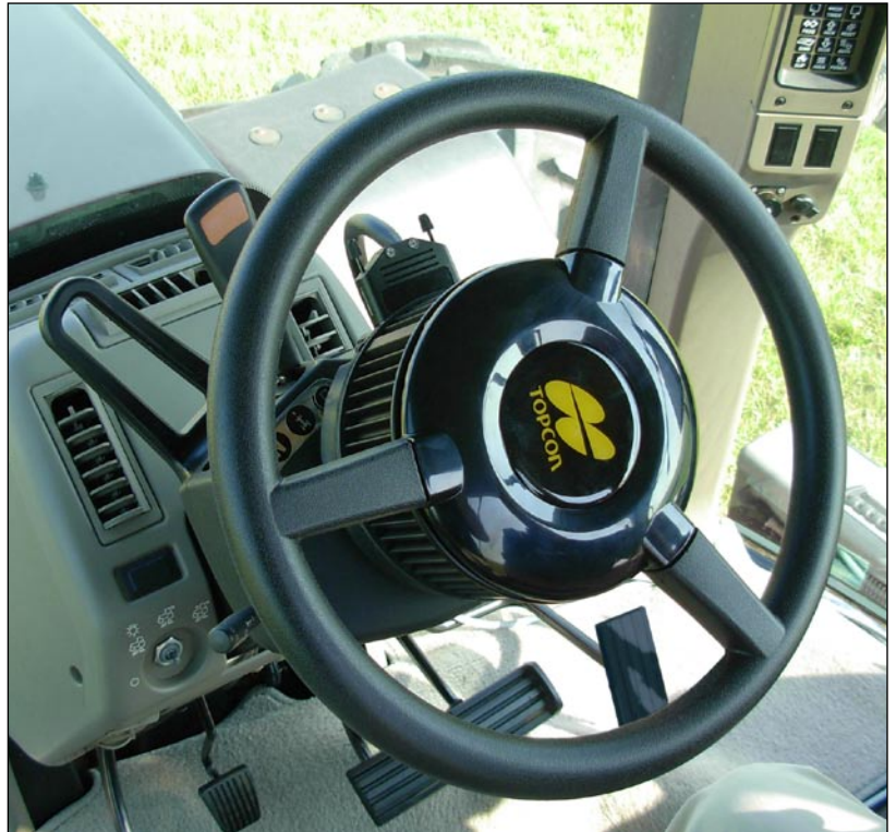
The AES-25 does not intrude into the operator's working area with external components that could interfere with normal day-to-day operation.
